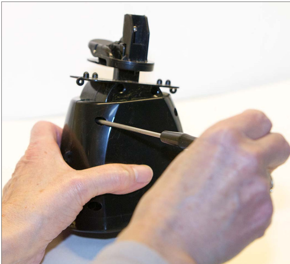
FIGURE 10-2: Removing the case of the movement mechanism.
