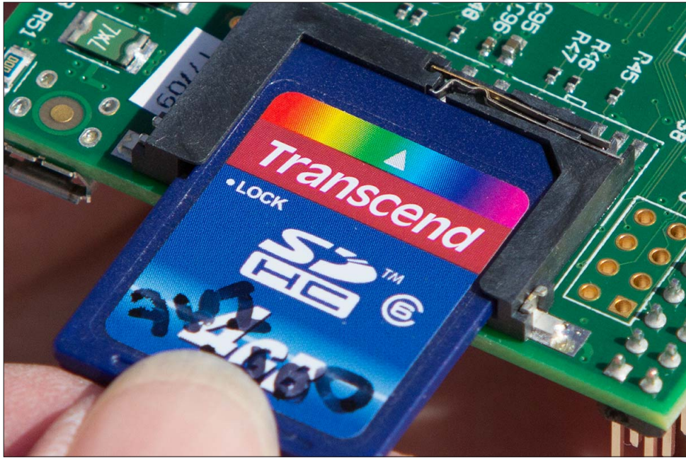
FIGURE 1-11: Take care not to snap off the plastic that keeps the SD card from falling out.
