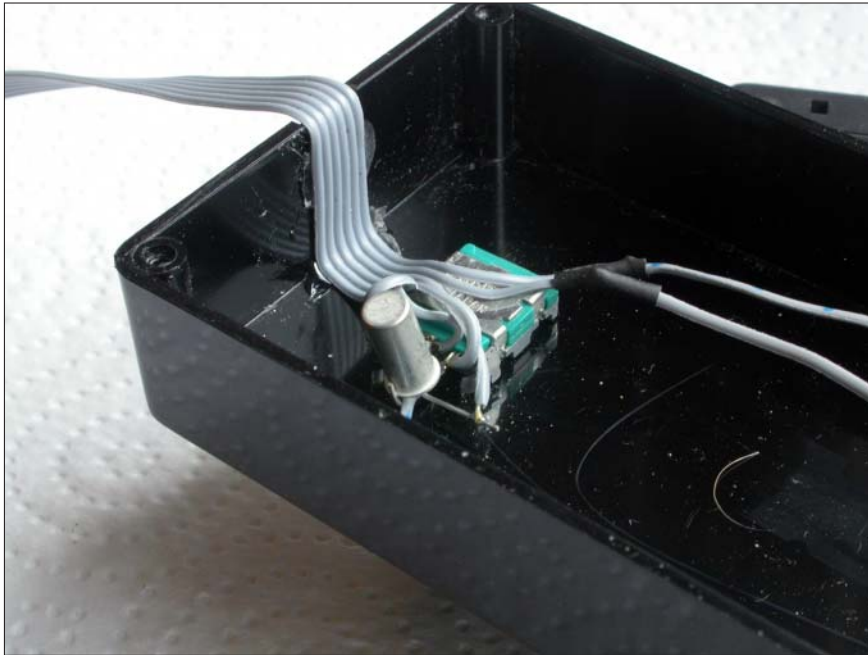
FIGURE 15-5: The wiring for the roto-sketch control box.
