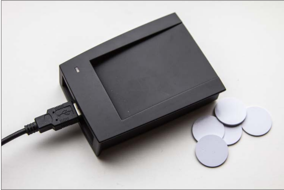
FIGURE 12-5: An RFID reader and tags.
