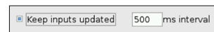
FIGURE 9-3: Enable the Keep Inputs Updated check box to show the status of inputs.
