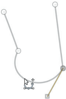
Figure 13.58 Moving a segment in nonpolygonal mode
