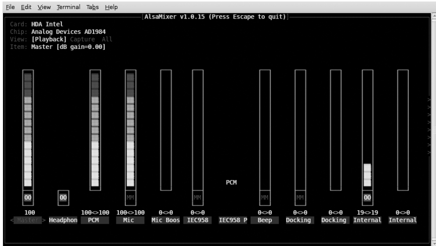
Figure 13-3: The alsamixer playback screen controls muting and volume on playback devices.
