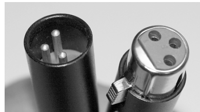
Figure 2-6: Here is a three-pin male XLR plug and a three-pin female XLR plug.
