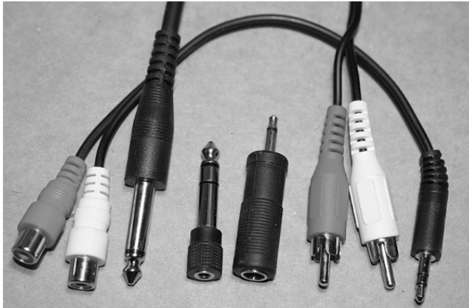
Figure 2-7: Two stereo RCA to 1/8" TRS plug, 1/4" mono TRS to two stereo RCA, 1/8" to 1/4" stereo TRS adapter, 1/4" to 1/8" mono TRS adapter
