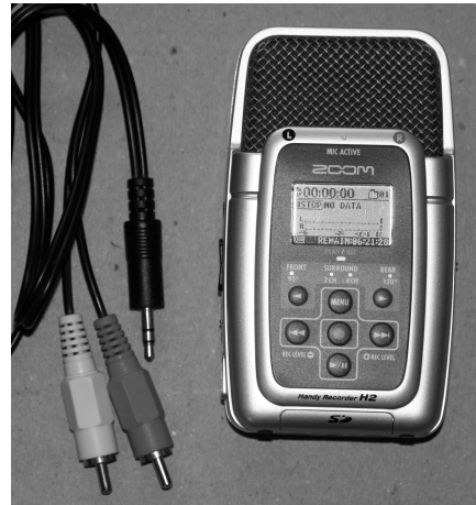
Figure 2-12: The Zoom H2 with an RCA-to-1/8" stereo plug adapter for connecting to a mixer or any other two-channel stereo RCA recording or line output
