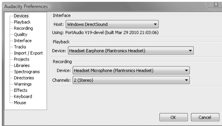
Figure 1-3: Select Edit > Preferences > Devices to set your default recording and playback devices.
