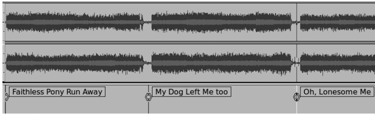
Figure 4-16: Creating song titles and breaking up a long track into individual songs with a label track
