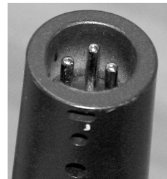
Figure 2-8: Behringer dynamic mic showing off its three-pin male XLR connector
