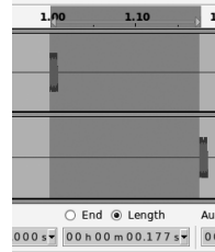
Figure 12-23: Measuring the latency between the two clicks on the click tracks
