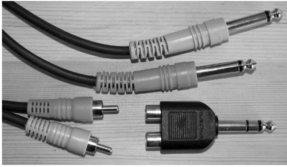
Figure 3-12: A two-RCA-to-two-1/4" TRS adapter. Note that the Y-adapter (bottom right) is not needed for connecting the MobilePre to the Record outputs on the amplifier. The Y-adapter comes in handy when I need to use a headphone jack for my recording source.
